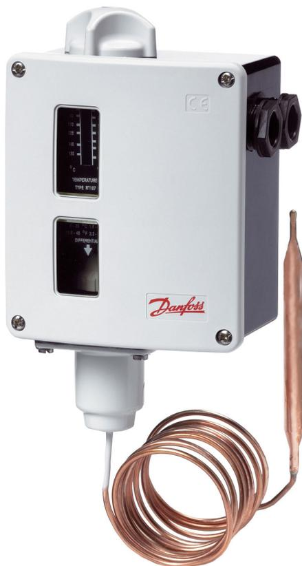
RT thermostats incorporate a temperature controlled, single-pole change over switch where the contact position depends on the temperature of the sensor and the set scale value.
