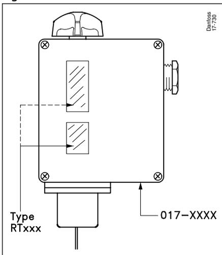
The type designation of the units is given on the setting scale. The code no. is stamped on the bottom of the thermostat housing.
